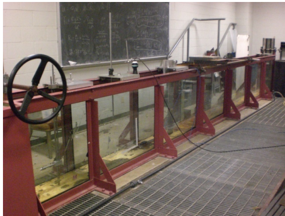
FIG. 5. A 25.5-ft long, 1.0-ft wide and 3.0-ft deep rectangular flume in the Hydraulic Lab
