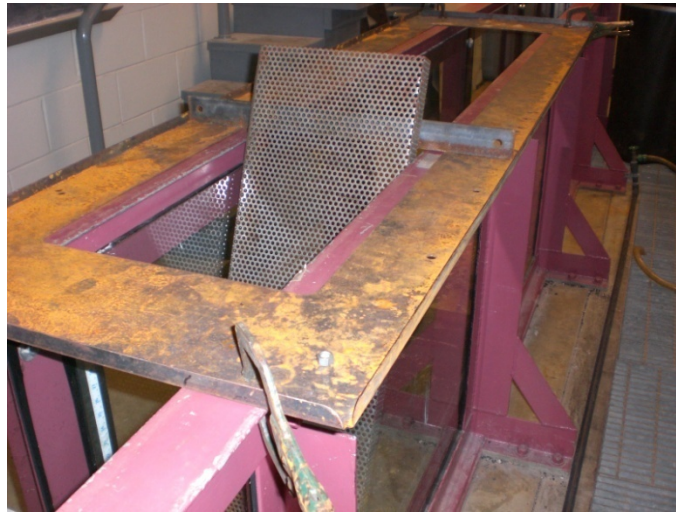
FIG. 11. Upper Brace Supporting the Porous Screen
